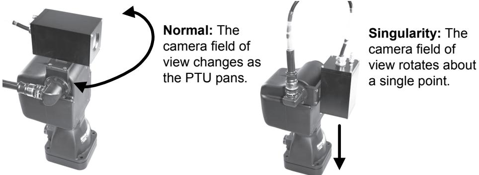
As the PTU approaches a singularity, the magnitude of pan motion required to correct for even small motions can become very large. Under some circumstances, the PTU will make continuous large pan motions as the payload pointing vector approaches +/-90 degrees.
