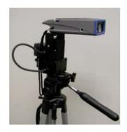
A data collection system for creating models for "as-built" models was developed by Dr. Yong Cho at the University of Nebraska (Cho and Haas, 2003). A laser range finder was integrated with a **Directed Perception PTU-D46 Pan-Tilt unit** to precisely position and record pan and tilt angles. The data was then compiled with the distance measurements to form a complete 3-D model.
